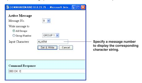
Example of Writing a Message (when the multi batch function (/BT2 option) is in use) Use message number 1 and write the message "start" to all display groups in batch group 1. Successful completion of the writing operation is indicated in the Command Response box.
